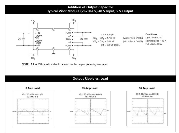
Figure 9–11 — Output noise, additional output capacitance
